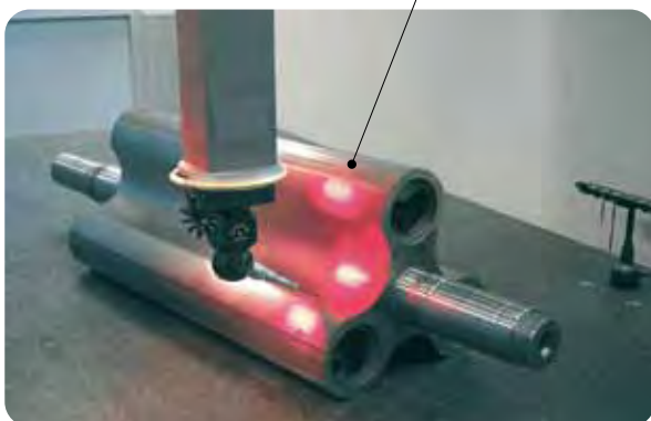
The grinding of the rotors and subsequent three-dimensional control ensure the highest performances.
