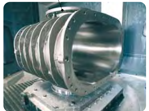
The precision milling and boring of the blower casing guarantee reduced tolerances and higher efficiency.
